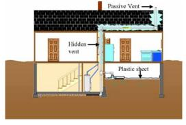
A smart contractor will route the vent pipe in such a manner that if, after the home is tested and the levels are not acceptable, a fan can easily be installed in the vent pipe within the attic to make the system more effective.
